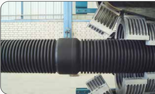
Production of NIC HDPE corrugated pipes with integrated socket
