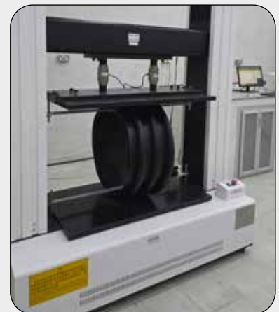
Ring stiffness testing as per ISO 9969
