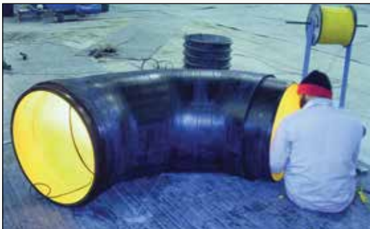
Bend for NIC HDPE Corrugated Pipe, with socket and spigot, for project in Iraq
